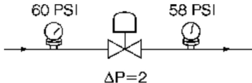
Figure 1: Pressure Drop Example
